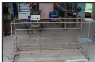
Basic frame work made from scrap. On skids to tow behind an ag bike.
